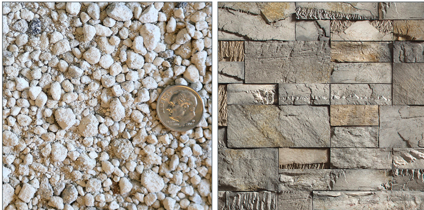
Left: HP Grade three-eighth x number 8 MN* (mine grade). Right: Grade used as an aggregate in lightweight stone, block, and brick veneers.
