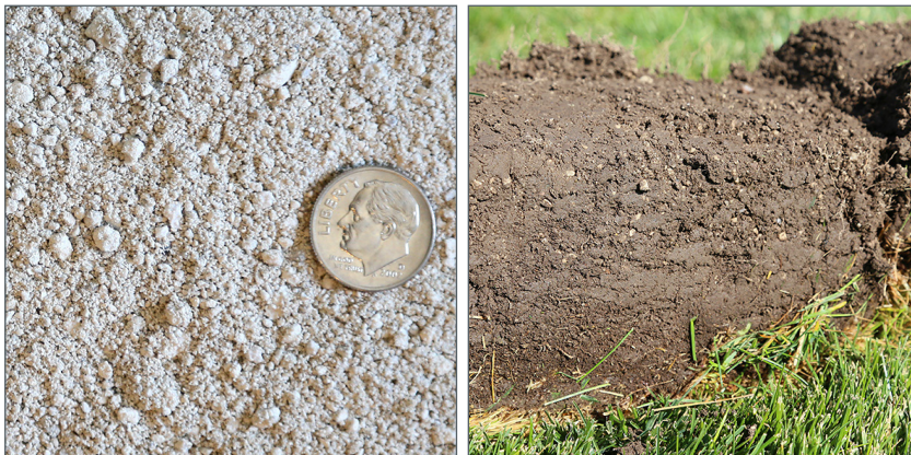
Left: HP Grade one-eighth fines MN* (mine grade) has a 1/8-inch top-end stone size with extensive fines content. Right: Grade used to amend heavy clay soil—improve root zone aeration, drainage and moisture retention, resist compaction—for a thriving lawn.
